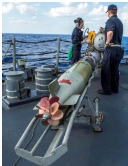
Torpeda ćwiczebna Recoverable Exercise Torpedo (REXTORP) Mk-46 Mod.5A
